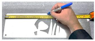
2 – Using the « Danger » imprint on the hopper as reference, mark the center line.
