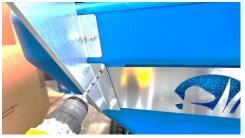
8 – Remove the bracket assembly, and install the support plate on the inside of the hopper. Note that flat washer should be used on the 2 top bolts.
