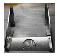
4 – Place the bracket assembly on the hopper.
