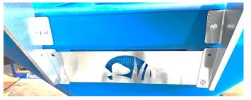
7 – Using the holes in the brackets as guides, drill the hopper.
