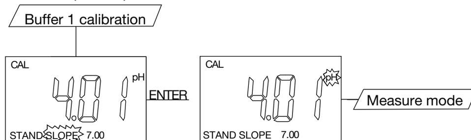
Rinse the pH and ATC/Temp probe in distilled water and immerse them in the second buffer solution (either 4.00/4.01 or 9.18/10.01). Allow temperature reading to stabilize, then press “ENTER” key to calibrate. The “pH” icon will flash until the unit detects a stable reading. Once the unit calibrates the second point and the unit will automatically exit the calibration mode and goes to the pH Measure mode. Dual point calibration is complete.
