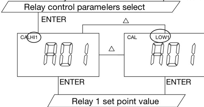
Pressing **[UP]** key or **[DOWN]** key in this screen will cycle the display from HI, LOW modes above. Select the preferred mode, press **[ENTER]** key to save, and enter the next setting screen.
