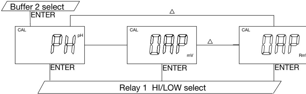
Pressing **[UP]** key or **[DOWN]** key in this screen will cycle the display from pH, ORP mV ORP RmV modes above. Select the preferred mode, press **[ENTER]** key to save, and enter the next setting screen.
