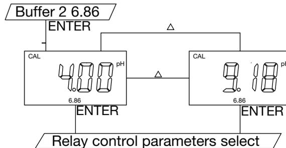
Pressing **[UP]** key or **[DOWN]** key in this screen will cycle the display from 4.01, 10.01 (or 4.00, 9.18) buffer above. Select the preferred buffer, press **[ENTER]** key to save, and enter the next setting screen.
