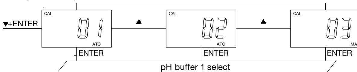
Pressing **[UP]** key or **[DOWN]** key in this screen will cycle the display from 01 (Thermistor: 10k ohm), 02 (Resistor: PT1000), 03 (Manual) modes above.
