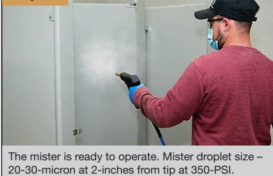
The mister is ready to operate. Mister droplet size - 20-30-micron at 2-inches from tip at 350-PSI.
