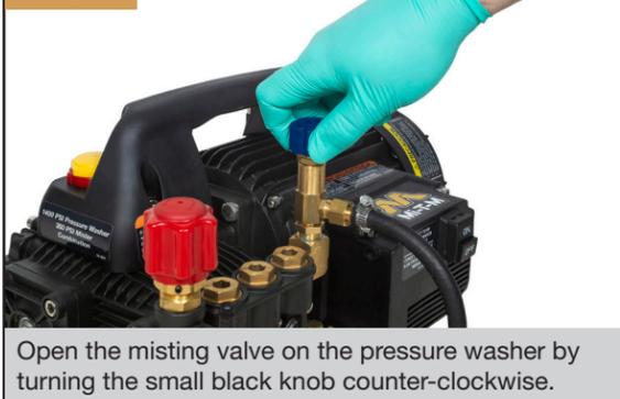
Open the misting valve on the pressure washer by turning the small black knob counter-clockwise.
