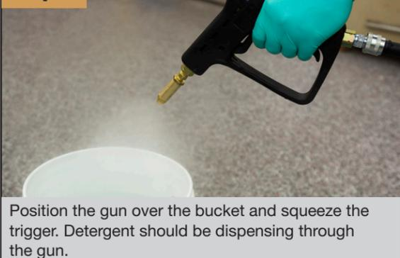
Position the gun over the bucket and squeeze the trigger. Detergent should be dispensing through the gun.
