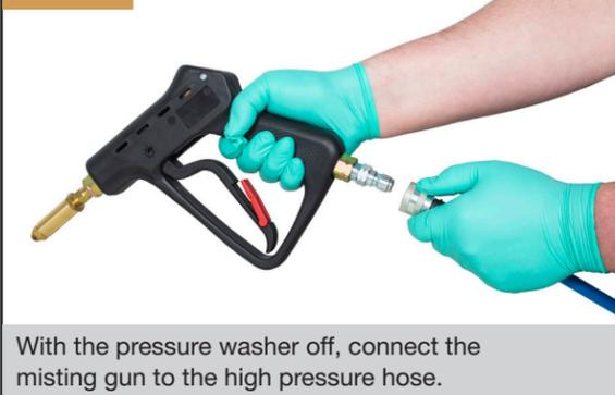
With the pressure washer off, connect the misting gun to the high pressure hose.
