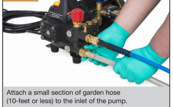
Attach a small section of garden hose (10-feet or less) to the inlet of the pump.
